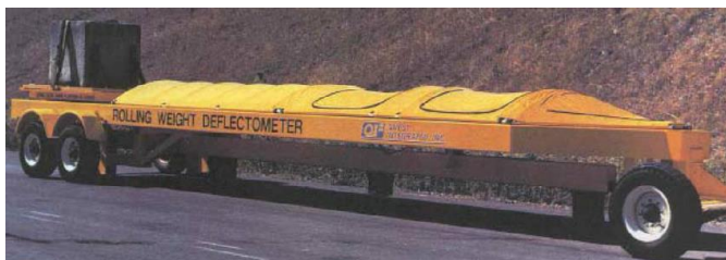
Airfield Rolling Weight Deflectometer by Quest Inc (US 1990's)
