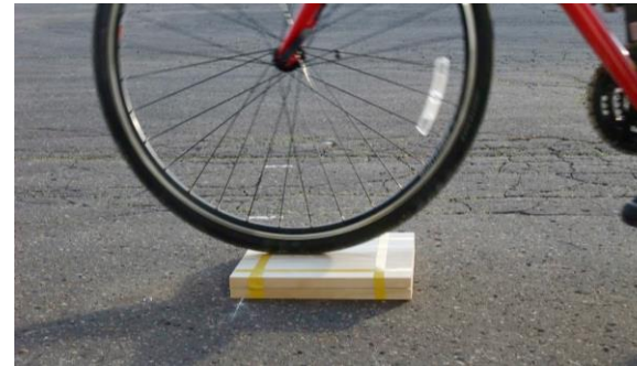
Ride Over Hump Test for Estimating Damping Ratio
