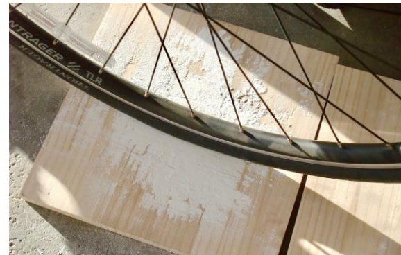
Measurement of Tire Envelope Length (150 mm)
