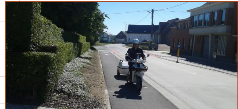
Bicycle path laser profiler of BRRC
